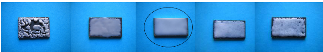
Fig. 4. Wettability of SACN glass on Crofer 22 APU using different SACN powder sizes ( d < 20 \mu\text{m} , d = 20\text{--}38 \mu\text{m} , d = 38\text{--}75 \mu\text{m} , d = 75\text{--}106 \mu\text{m} and d > 106 \mu\text{m} ) (25 °C/min, Ar).
